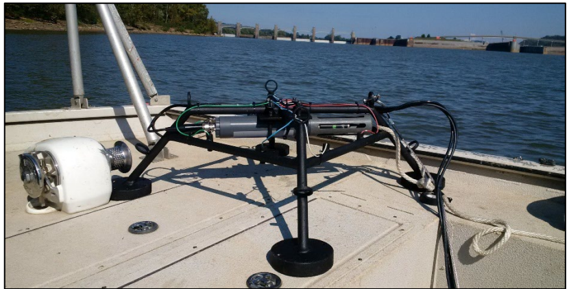
Figure 6. The WIZARD measures conditions in the actual substrate and the water column.
