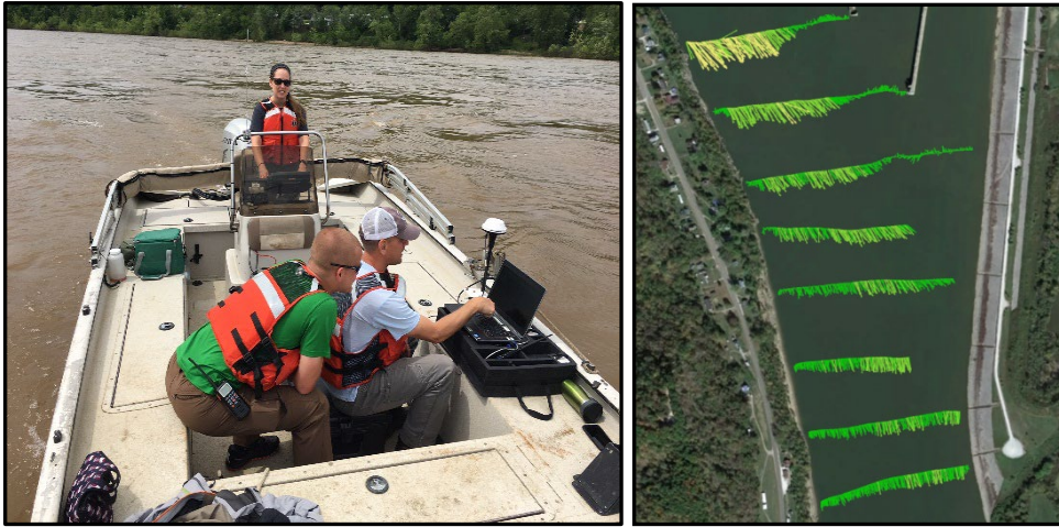
Figure 9. Velocity vectors demonstrating the effectiveness of steering currents employed below R.C. Byrd Dam.
