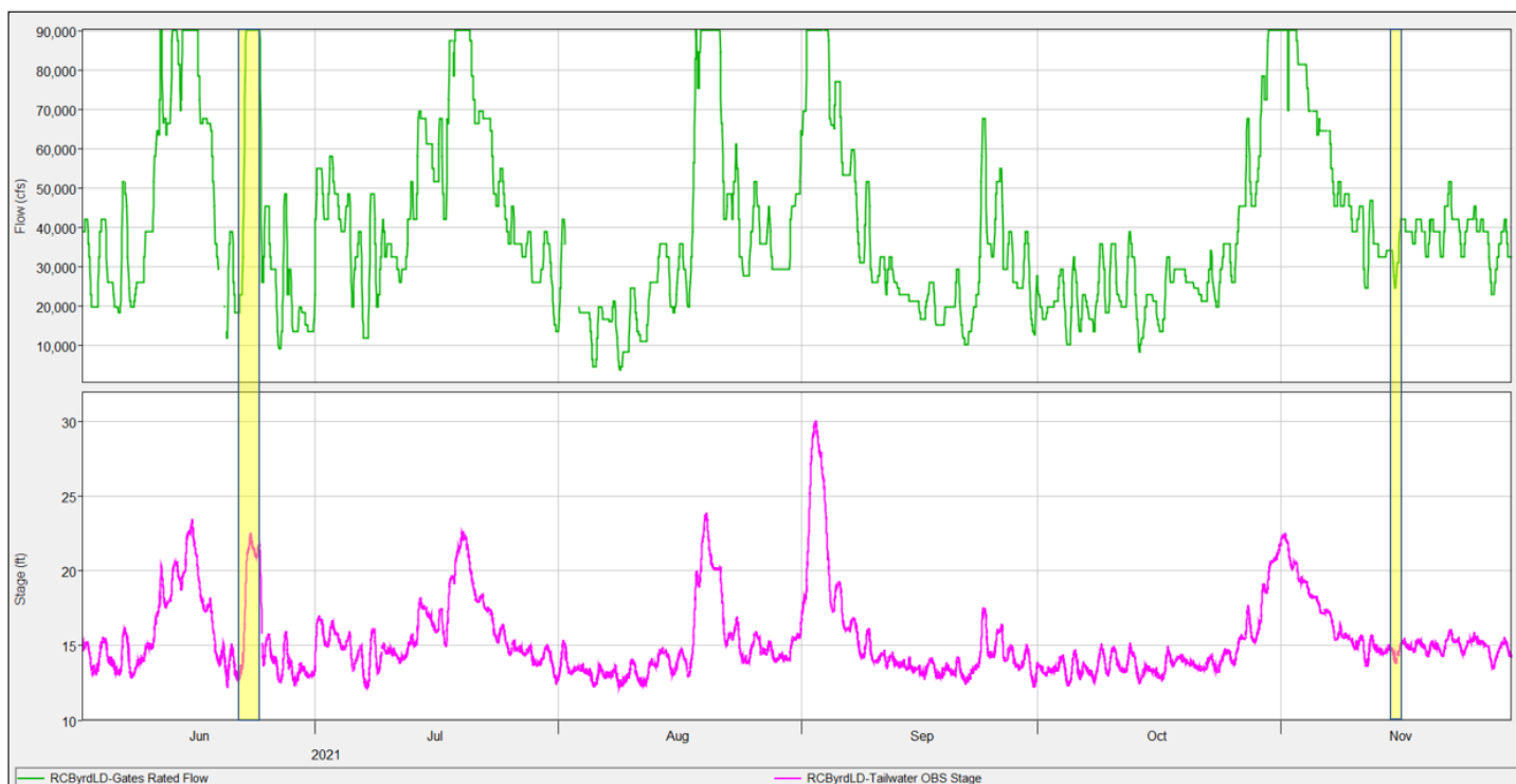
Figure 10. Flows, stages and dredge dates (yellow boxes) for R.C. Byrd dredging in 2021.
