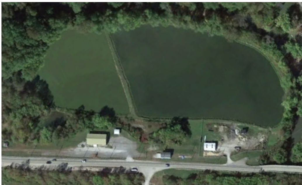
Figure 18. Lagoon #1 is on the left with an average sludge depth of 15.7 inches. Lagoon #2 is on the right with an average sludge depth of 3.1 inches.
