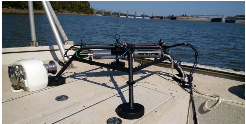
Figure 14. The WIZARD measures conditions in the actual substrate and the water column.
