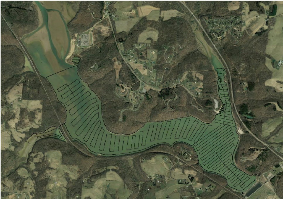
Figure 1. Bathymetry data collected using the EcoMapper and Acoustic Doppler Profiler.
